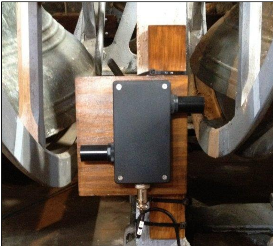
Figure 62 – Installed Sensor (Chirk, Type 1)
