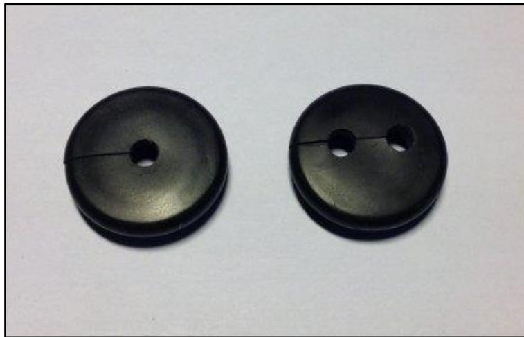
Figure 36 – Grommets Drilled & Cut
