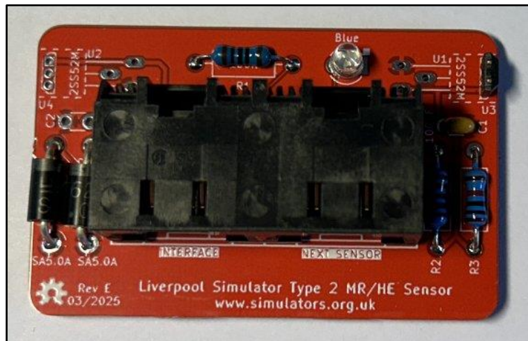
Figure 27 – Completed Magnetic Sensor Module PCB (A1120EUA-T, Right-Handed)
