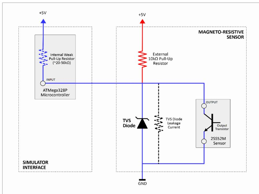
Figure 20 – Leakage Current – Supplementary Pull-Up Resistor
