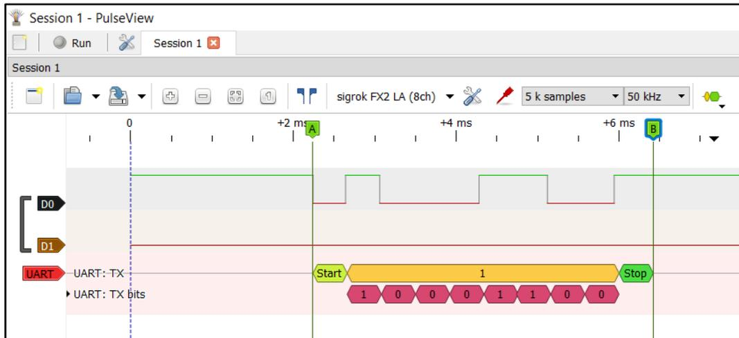
Figure 40 – Logic Analyser Decode
