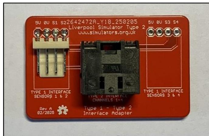
Figure 59 - Type 1 - Type 2 Adapter PCB
