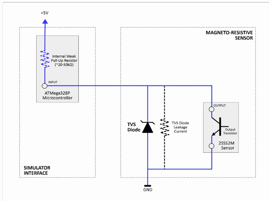
Figure 19 – Leakage Current "Voltage Divider" Effect
