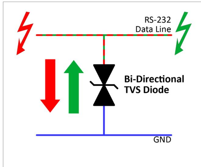
Figure 18 – Spike Dissipation (Bi-Directional)
