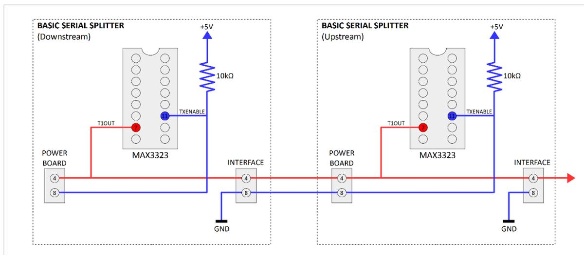
Figure 11 – Basic Serial Splitter Transmitter Control
