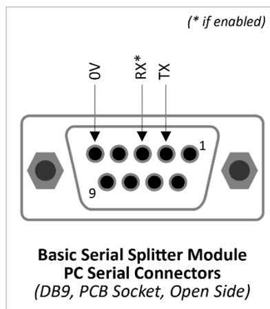
Figure 31 – Basic Serial Splitter DB9 Serial Connectors
