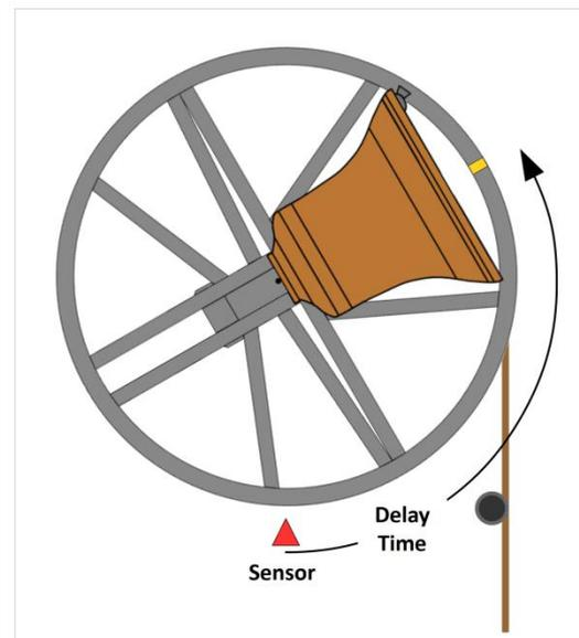
Figure 8 – Single Trigger – Handstroke Strike Point
