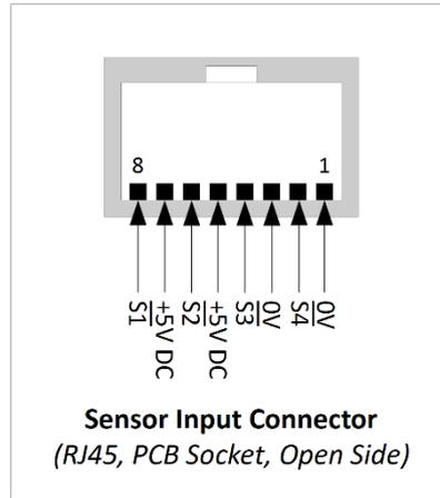
Figure 23 – Simulator Interface Module Sensor Connector
