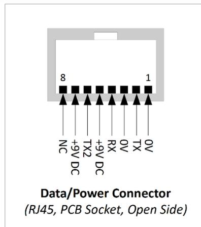
Figure 25 – Simulator Interface Module Power/Data Connector
