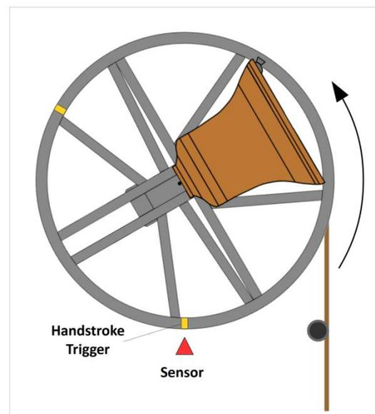
Figure 6 – Dual Triggers – Handstroke Strike Point
