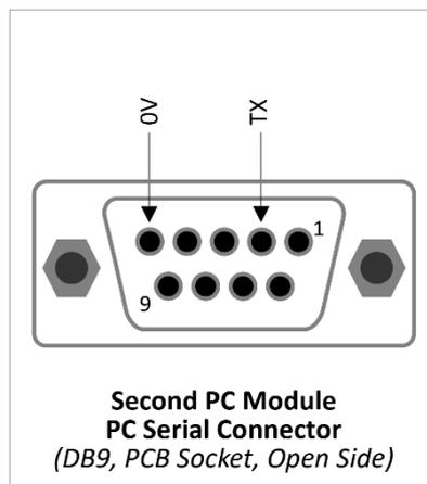
Figure 30 – Second PC Module DB9 Serial Connector
