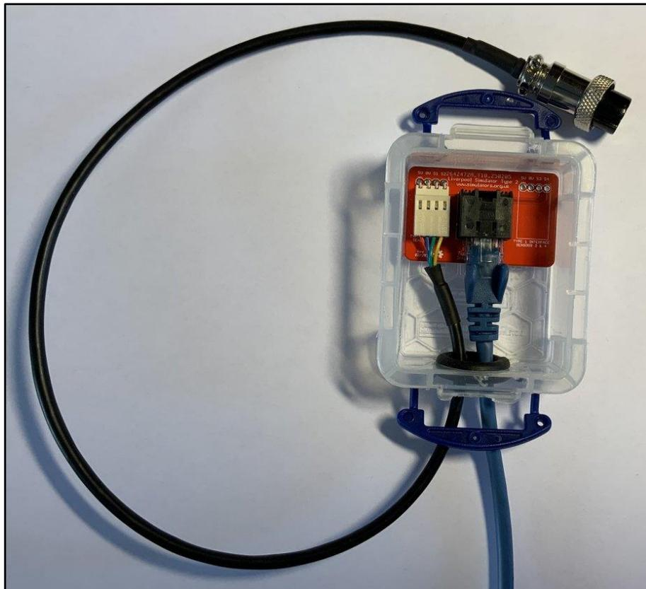
Figure 57 - Type 1 - Type 2 Adapter
