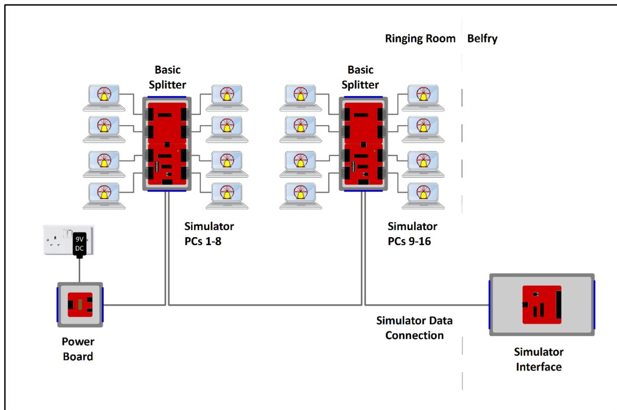
Figure 4 – Basic Serial Splitter Modules General Arrangement
