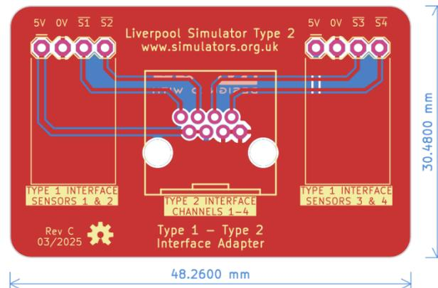
Figure 58 - Type 1 - Type 2 Adapter Board Layout
