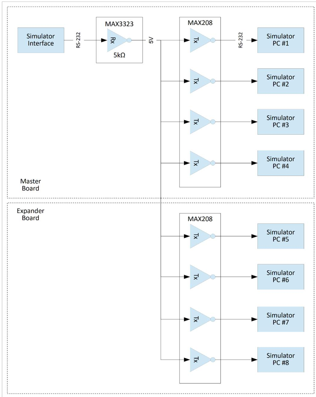
Figure 9 – Basic Serial Splitter Downstream Data Flow
