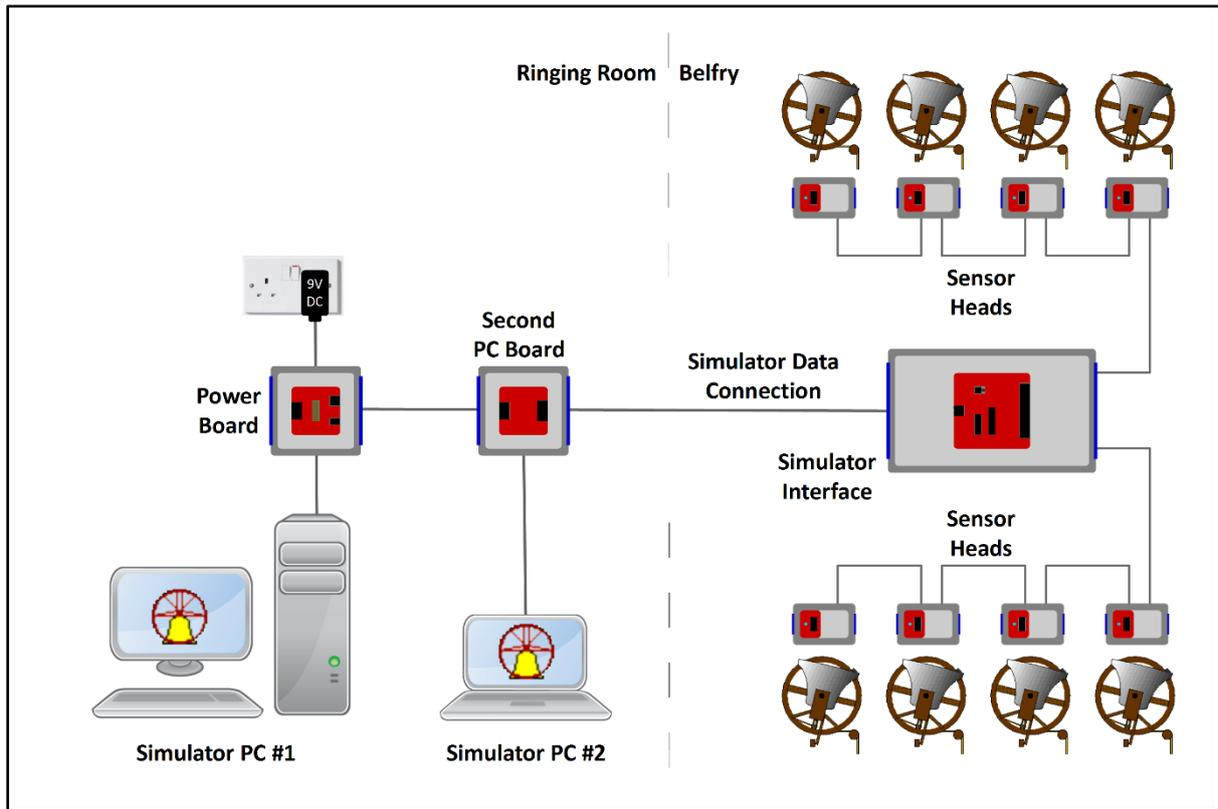
Figure 3 – Second PC Module General Arrangement
