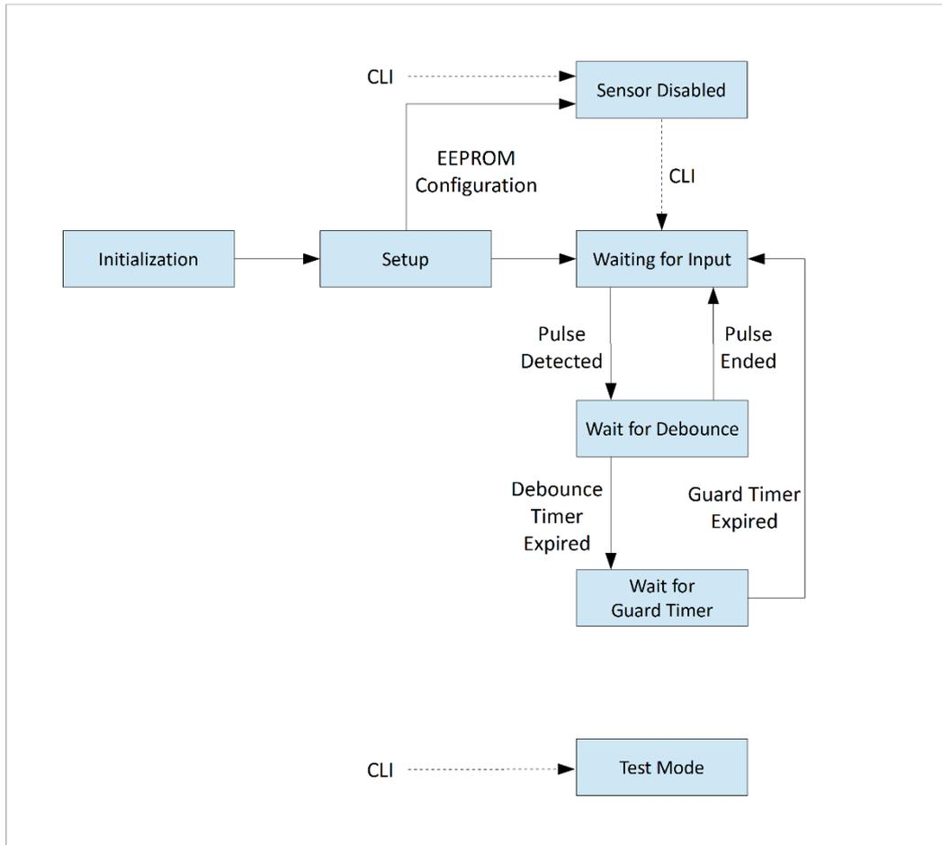
Figure 33 – State Machine Transitions Illustration
