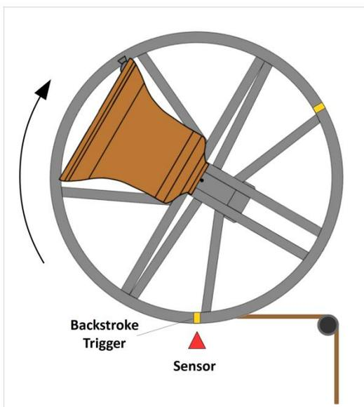
Figure 5 – Dual Triggers – Backstroke Strike Point
