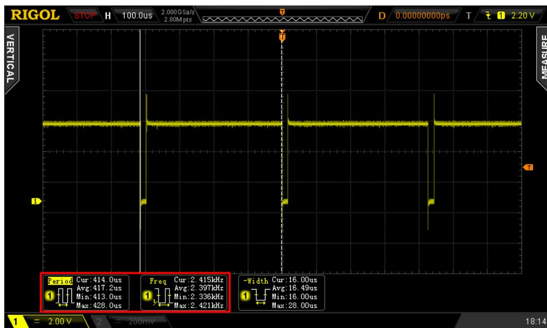
Figure 32 – Simulator Interface Main Loop Timing
