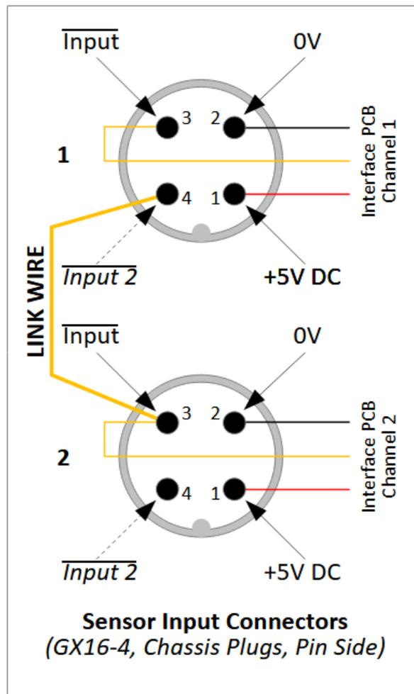
Figure 61 - Type 1 Interface Connector Wiring Modification
