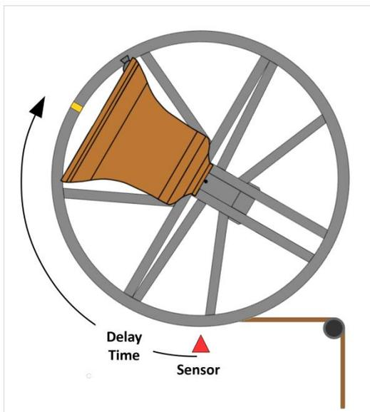
Figure 7 – Single Trigger – Backstroke Strike Point
