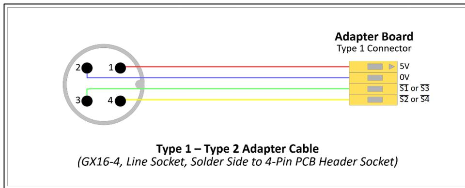
Figure 60 - Type 1 - Type 2 Adapter Cable
