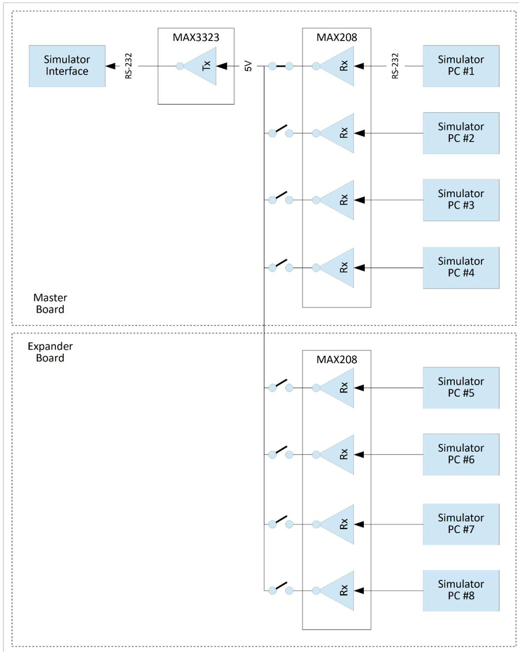
Figure 10 – Basic Serial Splitter Upstream Data Flow
