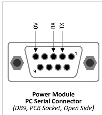
Figure 29 – Power Module DB9 Serial Connector
