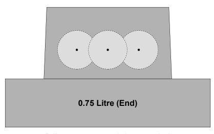
Drill centre or outer two holes as required.
